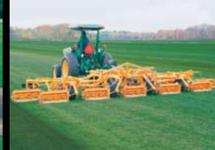
Kesmac 5, 7, 9 & 11 Gang Fixed & Floating Head Fairway Transportable Reel Mowers.
