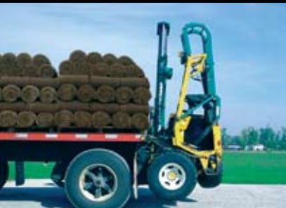
Kesmac Fixed and Retractable Leg Model Truck Mounted Forklifts. 4500 to 5500 lbs.
